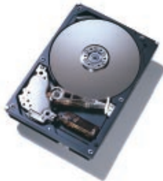
IBM Deskstar 75GXP 3.5-inch 7200 RPM 75, 60, 45, 30, 20, and 15 GB ATA disk drive
